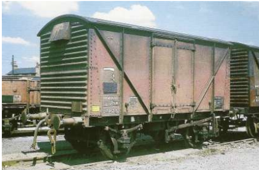
Illustrated above is the B.R. 12T Ventilated Plywood Van with, plain axle box and OLEO buffers.
