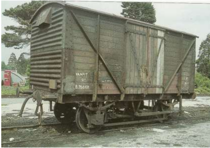
Illustrated above is the B.R. 12T Ventilated Van with planked doors, plain axle box and RCH buffers.
